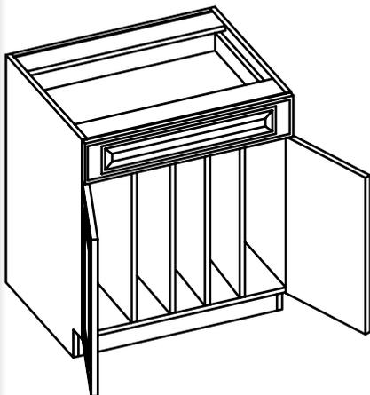
Tray Dividers for base cabinets. Made of 3/4" wood panels matching cabinet interior.
