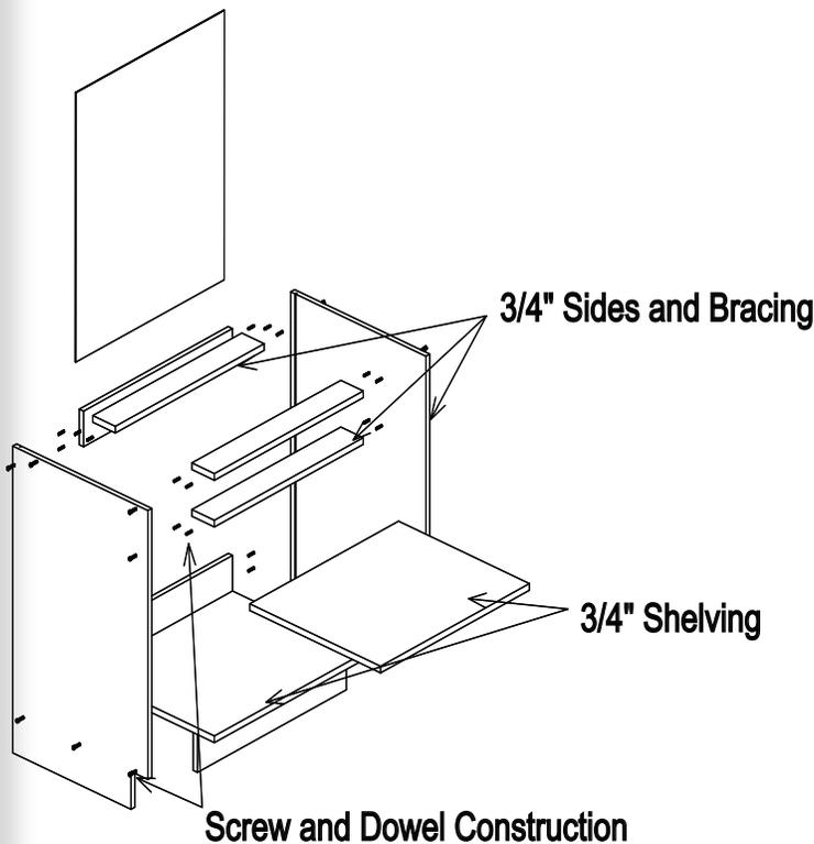
*3/4" material is used for all structural components, with screw and dowel construction, providing superior strength and rigidity.*
